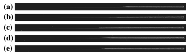
Fig. 7 Digitally scanned images of SAN 35 periodically scratch tested after being exposed to a humid environment, a dry, b 1 day, c 3 days, d 5 days, e 7 days (Resolution = 300 dpi, perpendicular orientation)
