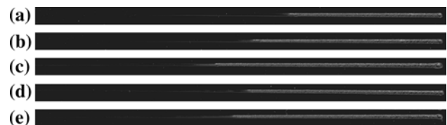
Fig. 6 Digitally scanned images of SAN 27 periodically scratch tested after being exposed to a humid environment, a dry, b 1 day, c 3 days, d 5 days, e 7 days (Resolution = 300 dpi, perpendicular orientation)
